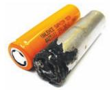
AA Batteries after a test in a 'Standard' Phi-TEC BTC
