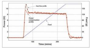
Comparison of heat-flow and power compensation profiles for water/acetic anhydride reaction
