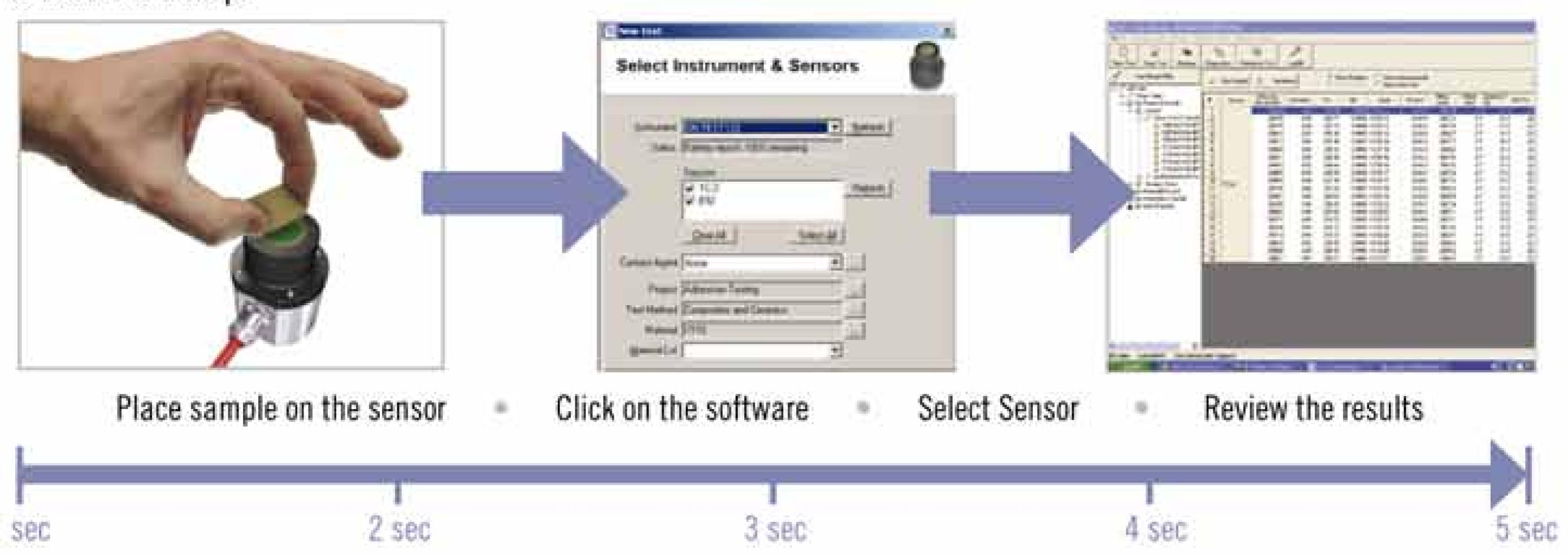
The C-Therm TCi features multiple graphical and tabular display options, and provides direct, indirect\* (calculated), and user input\*\* capabilities for a number of thermal testing properties, including:
